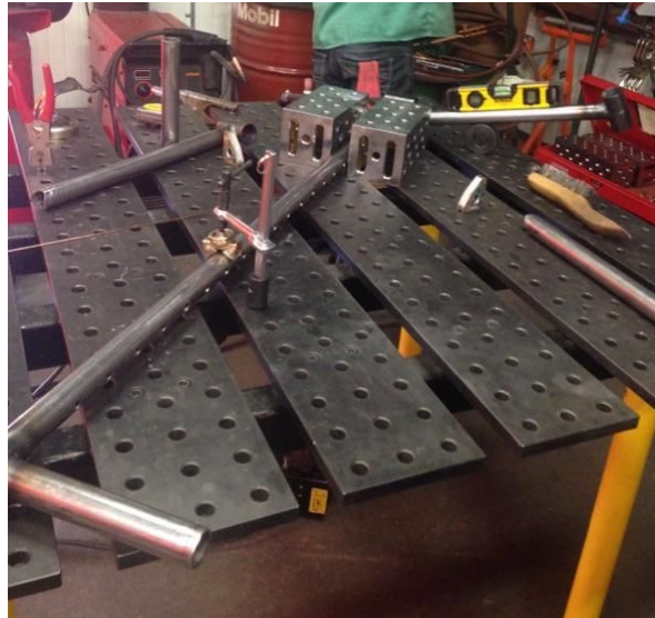
Figure 4: Side Arms Welding Configuration
